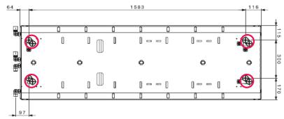
2 different bracket solutions according to the hydraulic connection and to the installation (vertical or horizontal) chosen by the installer
